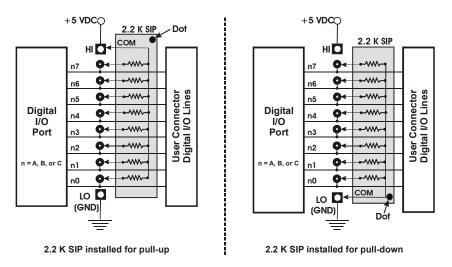
Figure 5. Pull-up and pull-down resistor SIPs schematic
